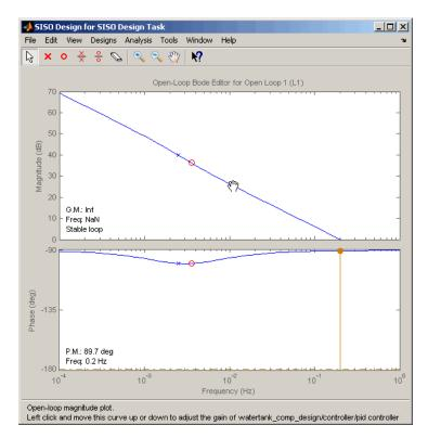
By increasing the gain, you increase the bandwidth and speed up the response. One possible compensator design that meets the tutorial requirements has the following parameters:
