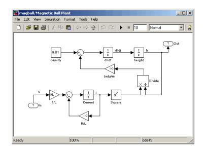
The Magnetic Ball Plant model represents an iron ball of mass M. This ball moves under the influence of the gravitational force, Mg, and an induced
