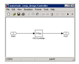
This model contains a PID Controller block that controls the height of the water in the Water-Tank System.
