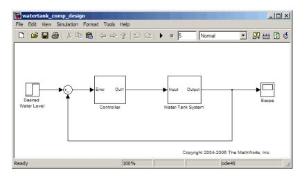
2 In the watertank\_comp\_design model window, select Tools > Control Design > Compensator Design. This action opens the Control and Estimation Tools Manager with the **Simulink Compensator Design Task** node selected.
